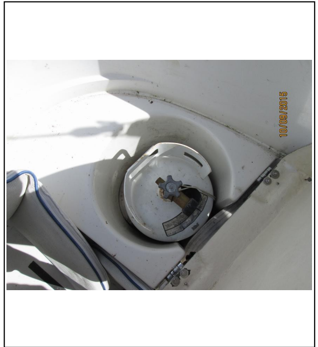
Spare tank locker.
