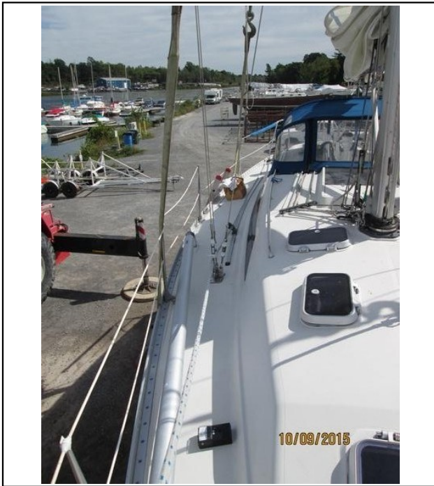
High moisture readings from meter aft to sheet winch.
