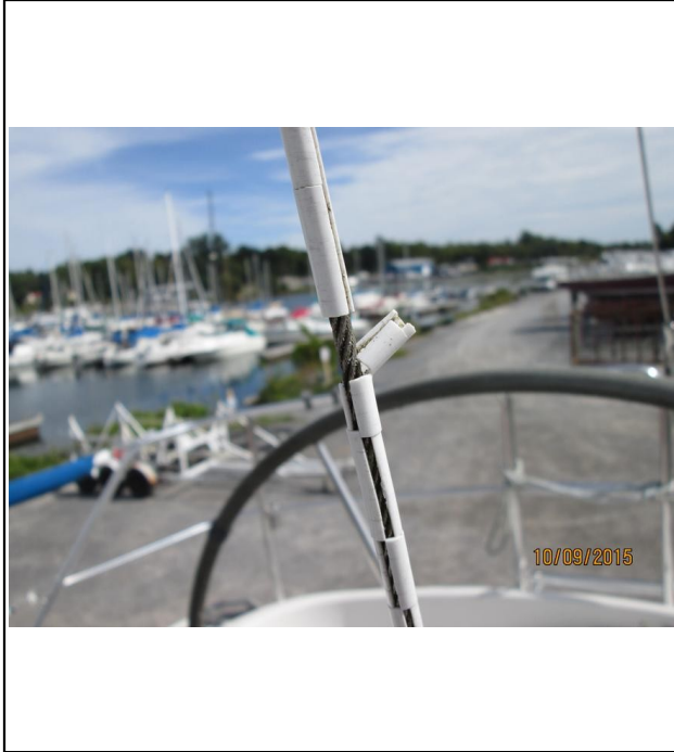
Cable attachment to main sheet.
